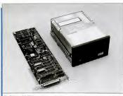
The Tallgrass TG-5525i is an easily installed internal hard disk that increases capacity by storing a whole track as a single long block of information.
